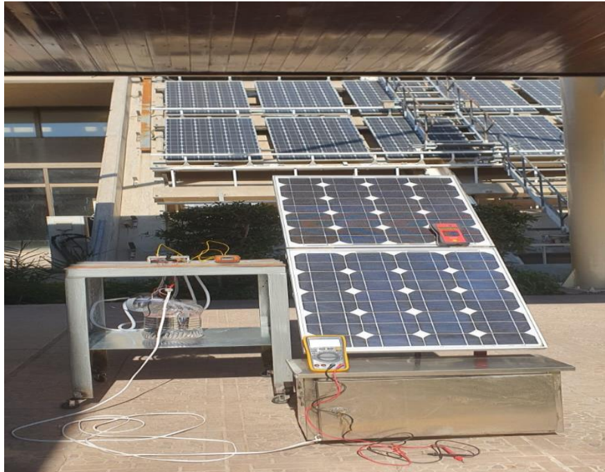
Figure (3): The implemented Seebeck system during testing a sample (p-type silicon).
