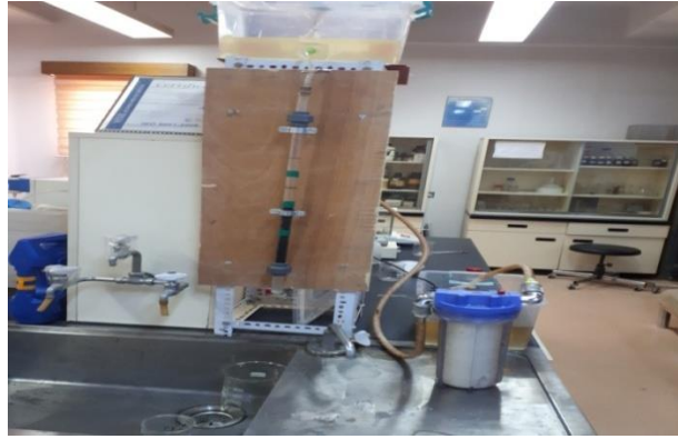
Figure (2): Filtration and carbon fixed bed column of treatment.
