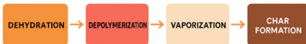
Figure (2): Thermal decomposition stages of cellulose Created by authors.
