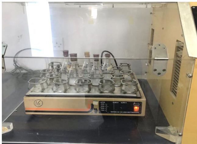
Figure (2): The adsorbent and the adsorbate during the batch adsorption analysis in the shaker.
