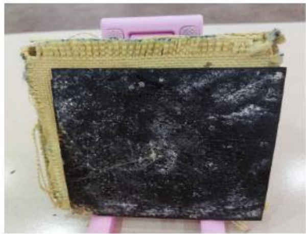
Figure (13): Tested samples of Bullet Test with 2MPa pre-stressing fiber and 1wt.% Nanographene.
