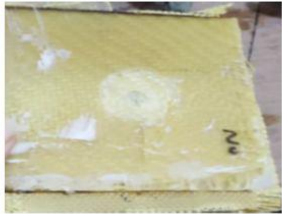
Figure (11): Tested sample of Bullet Test with prestressing fibers of 2MPa without Nanographene.
