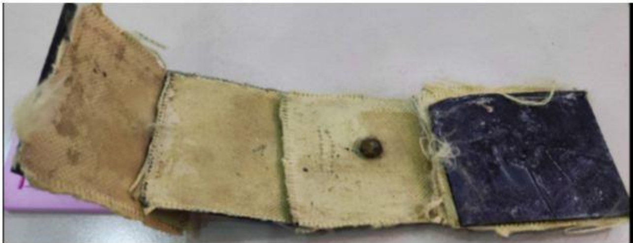
Figure (14): Tested sample of Bullet test with 2MPa pre-stressing fiber and 2wt.% Nanographene.
