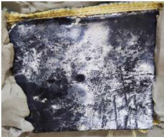
Figure (12): Tested sample of Bullet Test with prestressing fibers of 2MPa and 0.5wt.% Nanographene.
