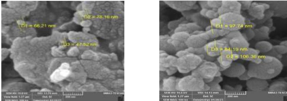
**Figure (5).** Scanning electron microscope analysis of heat treatment carbon-sulfur samples extracted by NaOH solution.
