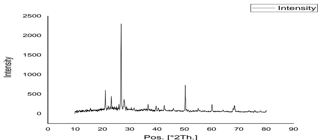
**Figure (8).** X-ray diffraction pattern of carbon-sulfur compounds air-thermal heat treated at 160-170 °C.
