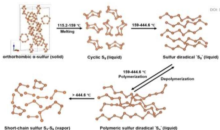
**Figure (4).** Structural transitions of elemental sulfur at different temperatures.
