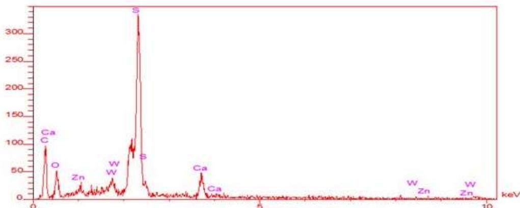
**Figure (3).** The energy spectrum of the dispersive X-rays (EDS) of carbo-sulfur materials extracted from foam.
