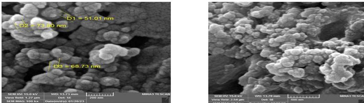
**Figure (2).** Scanning electron microscopy (SEM) analysis of the carbo-sulfur materials extracted from foam.
