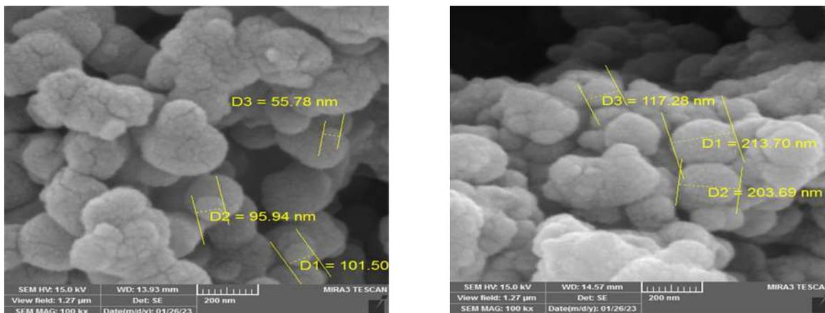
**Figure (6).** Scanning electron microscope analysis of carbon-sulfur samples for air-thermal treatment extracted by NaOH solution.
