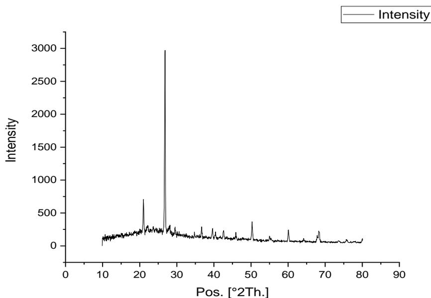
**Figure (7).** X-ray diffraction pattern of carbon-sulfur compounds heat treated at 160-170 °C.
